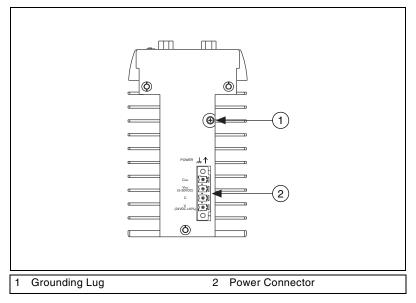
Figure 3-5. Grounding Lug on the CVS-1450 Device
